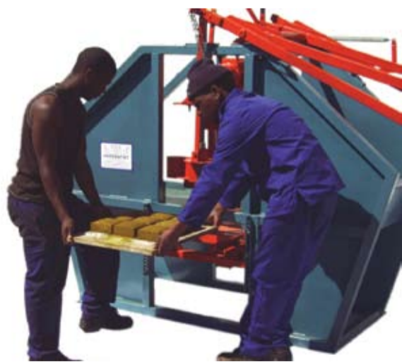
The Hyperstat can manufacture stock bricks, maxi-bricks, face bricks, rock-face or patterned decorative bricks. It can produce solid blocks, cavity blocks of all shapes and dimensions, retaining wall blocks, curb stones, lock blocks, deck blocks, face blocks, interlocking blocks, as well as wind-blocks.
