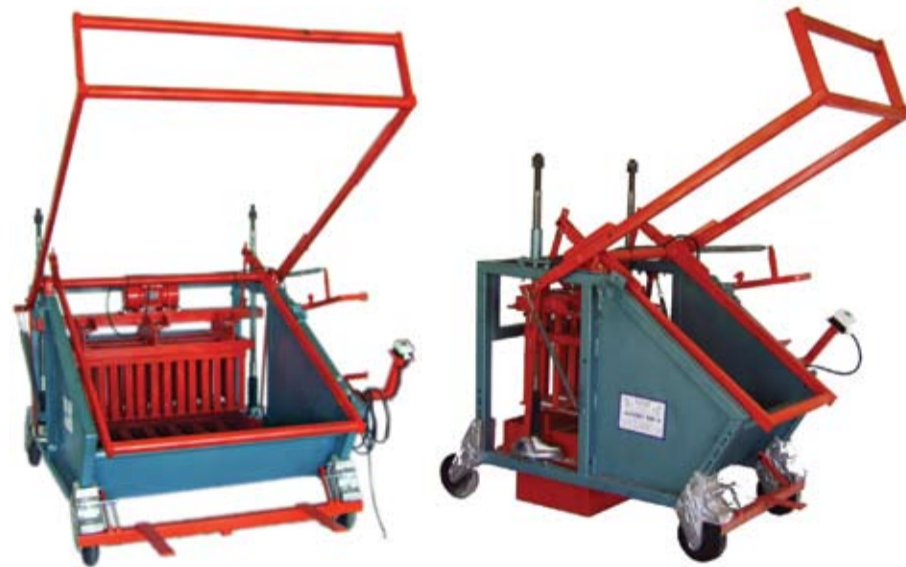
The Doubell Jumbo MK II (left) brick machine has a worldwide reputation for being easy to use while producing a quality product. The Doubell Jumbo MK III (right) has built on this reputation through been a larger machine thereby producing more product in the same amount of time. It can accept over 33 different interchangeable moulds as well as infinite custom built moulds that can be made to suit customer requirements. It uses the same basic principles as the MK II and thus has a cycle drop time of around 25 seconds.
